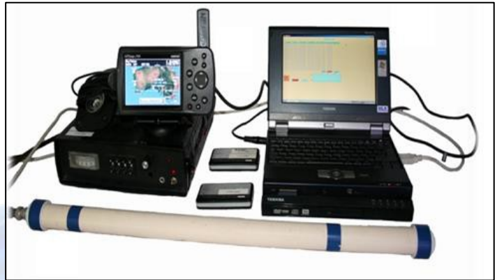
Figure 7: The AEM-PTP survey equipment to be installed in the aircraft
